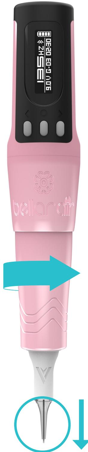
*Turning the grip as shown increases needle depth.*
