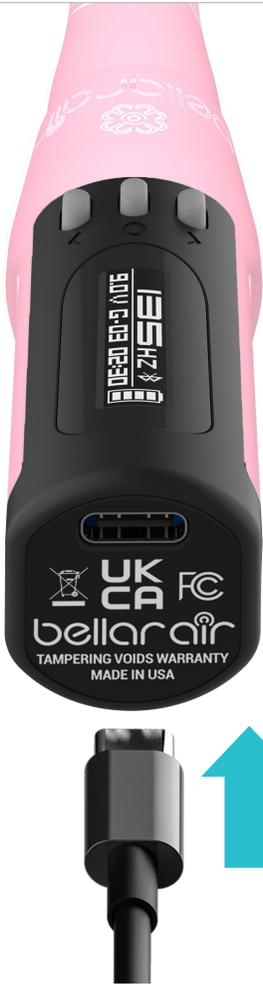
1 Plug the USB-C cord into the battery connector.
